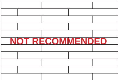
Brick bond installation 50% (NOT RECOMMENDABLE)
